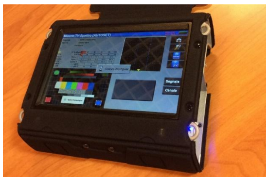
Figure 4-6: Sefram 7876 installer meter.
