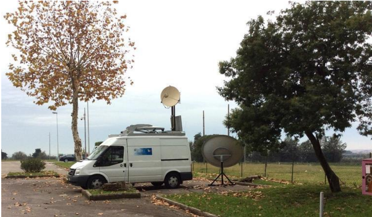
Figure 3-2: VSAT receiver dish, with MISE van used for field-strength measurement
