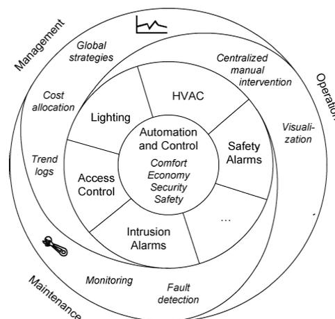
An important driver to this integration is the development of wireless technologies, thus enabling new applications to be deployed and releasing the immense potential of integrated systems. Wireless building automation (WBA) involves the introduction of the use of wireless networking technologies in the management of public buildings or professional infrastructures. There is a whole range of technical equipment that could be included within this network:
