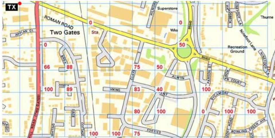
Figure 4.4b: Measured %-location coverage (Two Gates)
