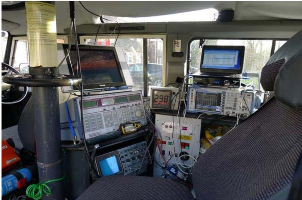
**Figure 3.10: Internal arrangement of Aegis measuring vehicle**
