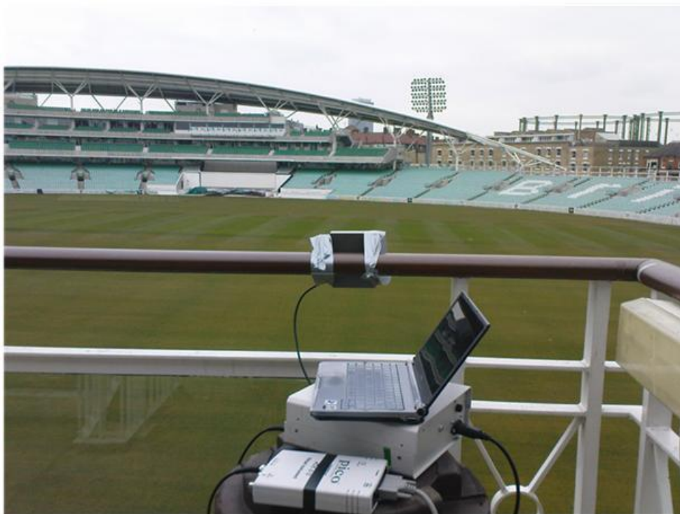
Figure 5.6: Canopy generating long-delay reflections in stadium
