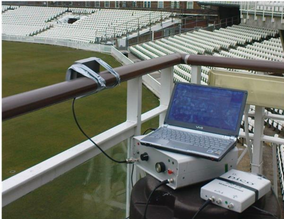
Figure 5.2: Aegis channel sounder (receiver)
