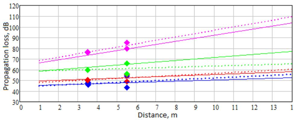
Figure 8.10: Data and model, modern terraced house
