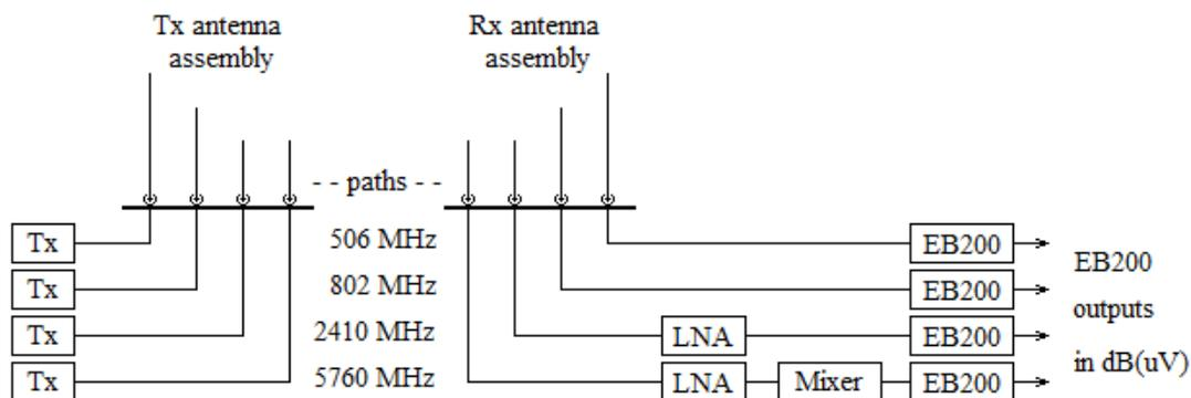
Low-noise amplifiers precede the EB200 measuring receivers for the upper two frequencies. A down-converting mixed is also needed at the highest frequency.
