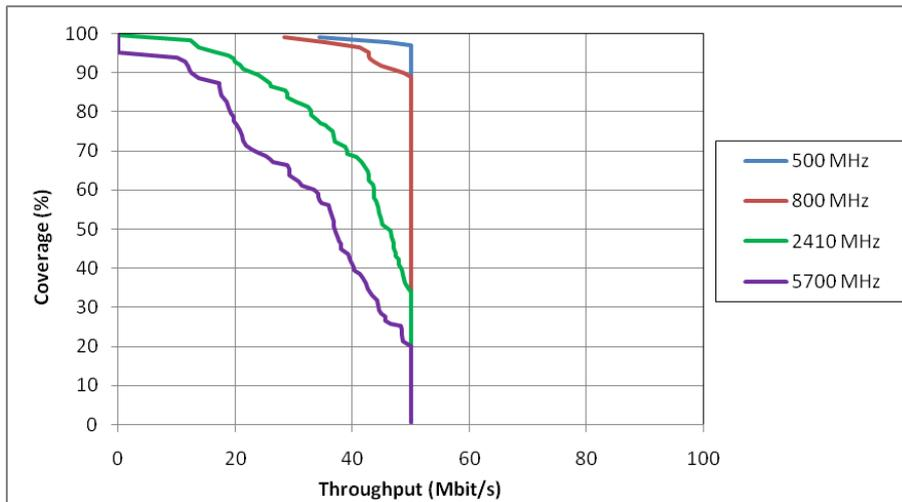
Figure 9.11: Predicted coverage distribution, UK weighted average, MIMO
