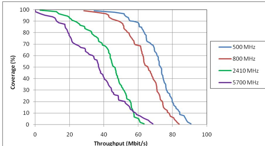
**Figure 9.13: Predicted coverage, UK weighted average, MIMO extrapolated**
