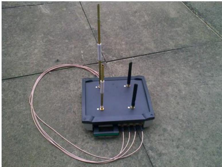
The antenna unit consists of four dipoles, two of which (for 2.4 GHz and 5 GHz) are commercial items while those for the lower frequencies were built at RAL.
