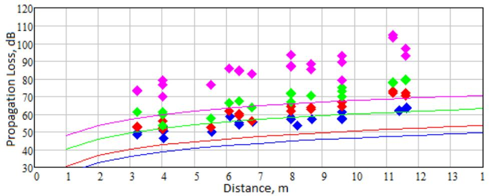
Figure 8.4: Modern detached house, same-floor measurements
