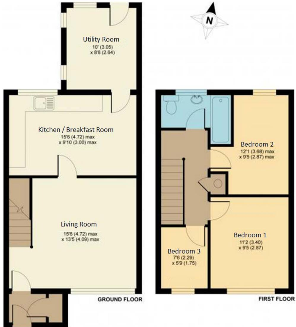
In this house only one hub location was used. This was in the living room, located 0.85 m from the E wall and 0.65 m from the window in the S wall. This was near the main ADSL connection point. The antenna height was 1.2 m.
