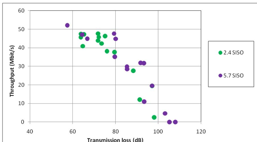
**Figure 9.5: Throughput scatterplot, Victorian terraced house, MIMO**
