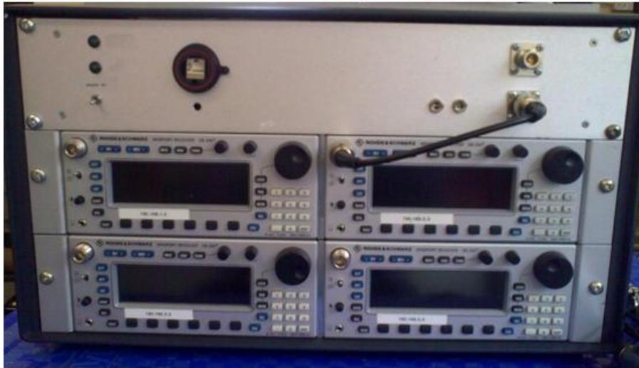
The receivers are controlled over an Ethernet interface by a PC running Aegis Systems 'Logger' software.
