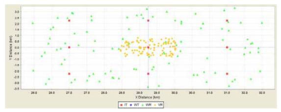
Figure 4: Mobile WiMAX BS TX into DTT RX Interference Scenario Outline from SEAMCAT (DTT RX at DTT Coverage Edge)
