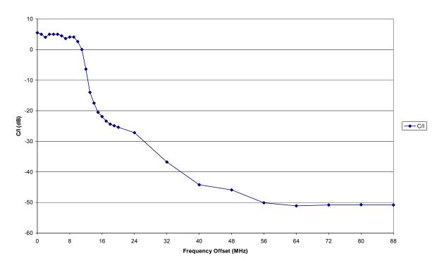
Figure 22: Extended C/I protection ratios for DTT into WiMAX
