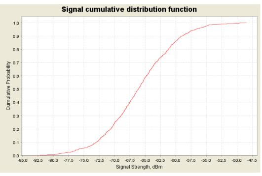
Figure 10: Wanted Power CDF at DTT RX (Mean = -66.1 dBm, Std Dev = 5.63 dB)
