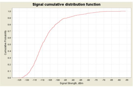
Figure 11: Interference Power CDF at DTT RX (Mean = -107.53 dBm, Std Dev = 10.58 dB)
