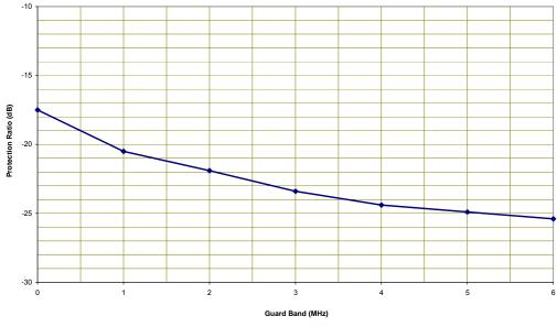
The following figure illustrates the measured protection ratios (by ERA) as a function of guard band between the DVB-H TX and mobile WiMAX SS RX channels.
