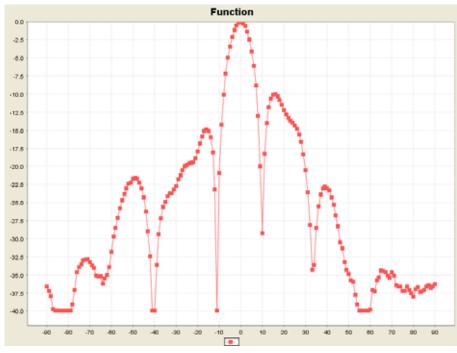
Assumed mobile WiMAX BS RX antenna vertical and horizontal patterns are shown in figures below.
