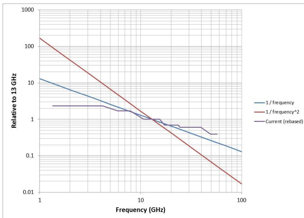
Source: Aegis analysis relating frequency to distance and distance squared assuming 13 GHz to be the reference point (i.e. equal to 1)
