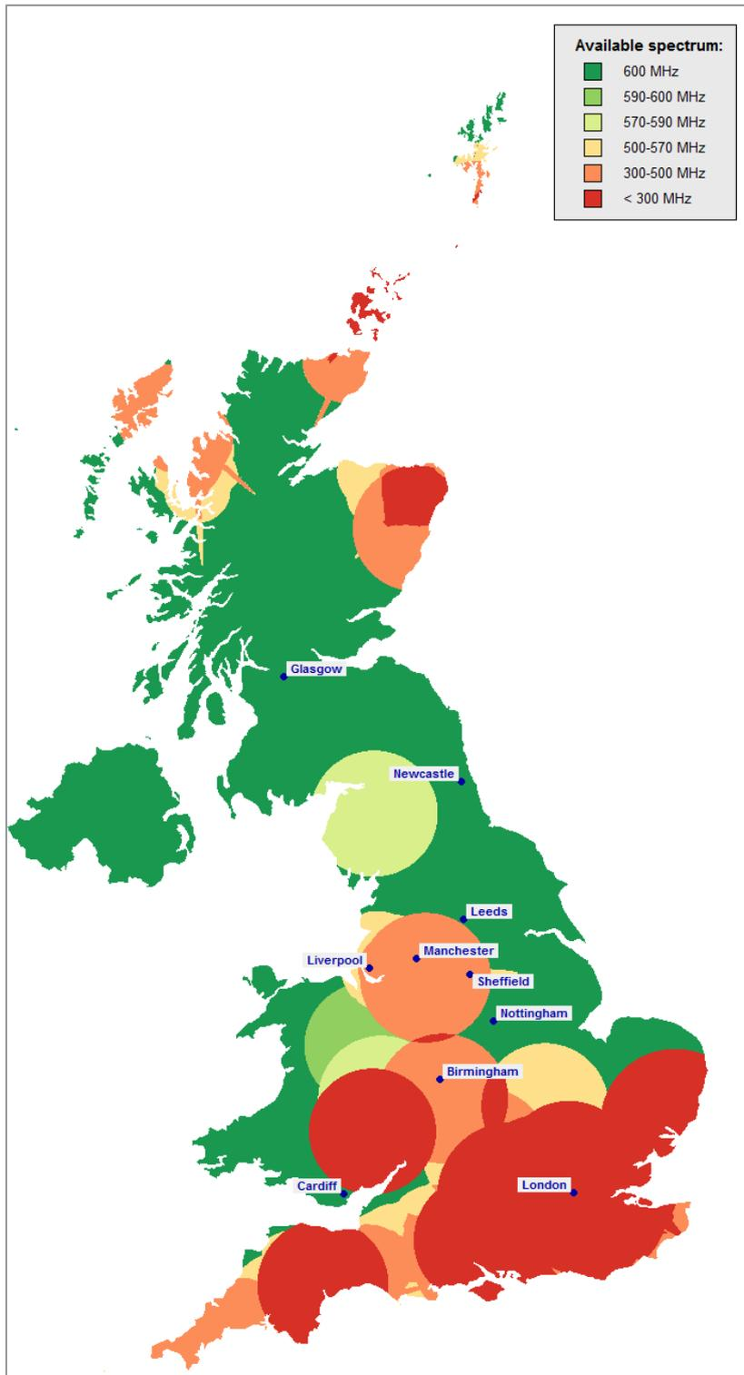
Figure A-16: Amount of spectrum (within the 3600 – 4200 MHz range) that could be available for IMT small cell use outdoors within the coordination areas around earth station receivers based on ITU-R criteria
