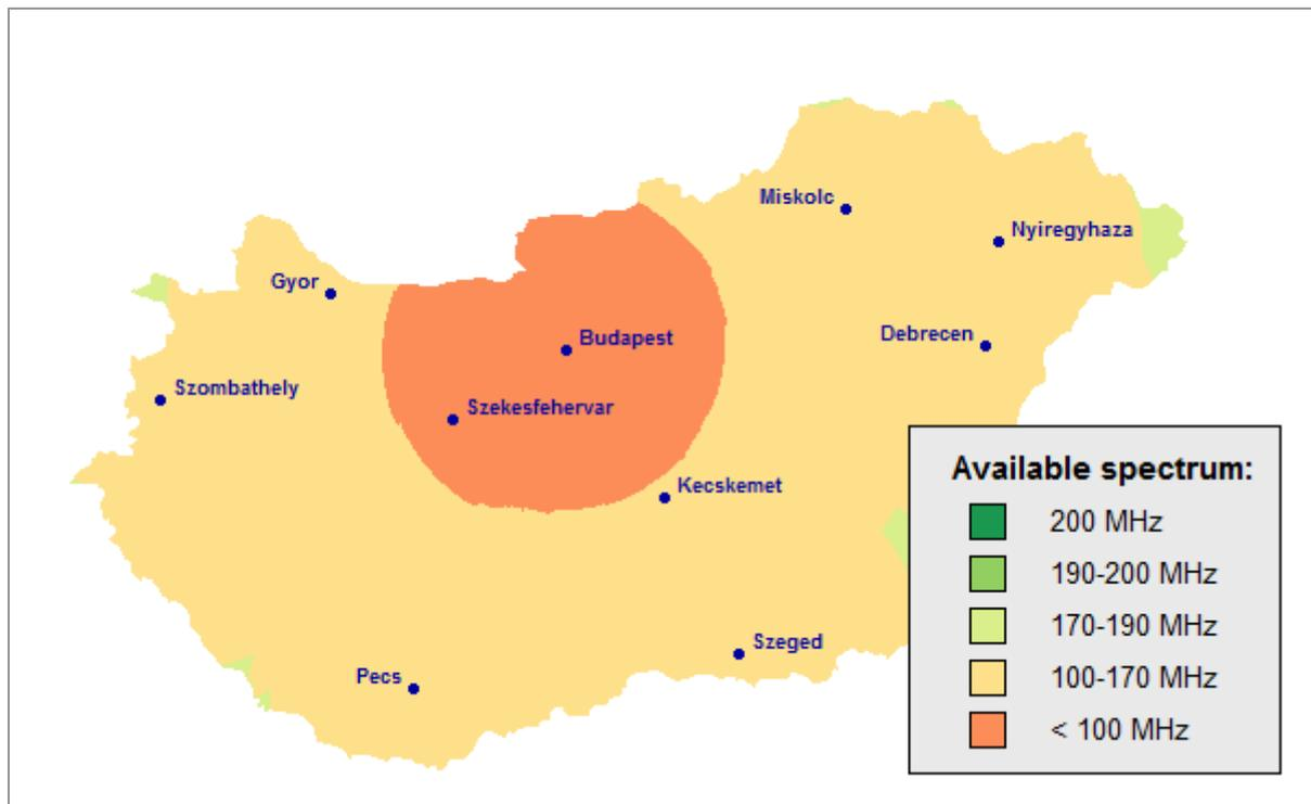
Figure A-2: Amount of spectrum (within the 3400 – 3600 MHz range) that could be available for IMT small cell use within the coordination areas around fixed link receivers (P-MP base stations) based on ITU-R criteria
