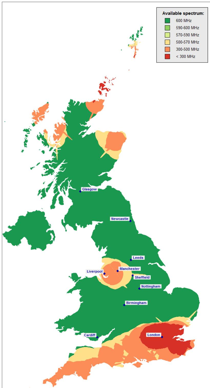
Figure A-15: Amount of spectrum (within the 3600 – 4200 MHz range) that could be available for IMT macro-cell use within the coordination areas around earth station and fixed link receivers combined based on ITU-R criteria
