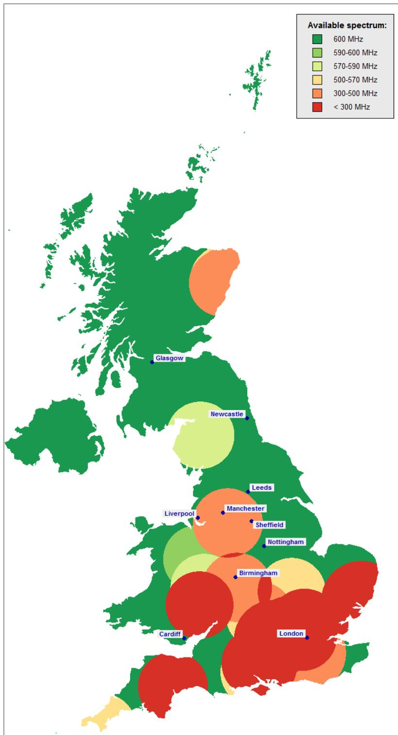
Figure A-14: Amount of spectrum (within the 3600 – 4200 MHz range) that could be available for IMT macro-cell use within the coordination areas around fixed link receivers based on ITU-R criteria
