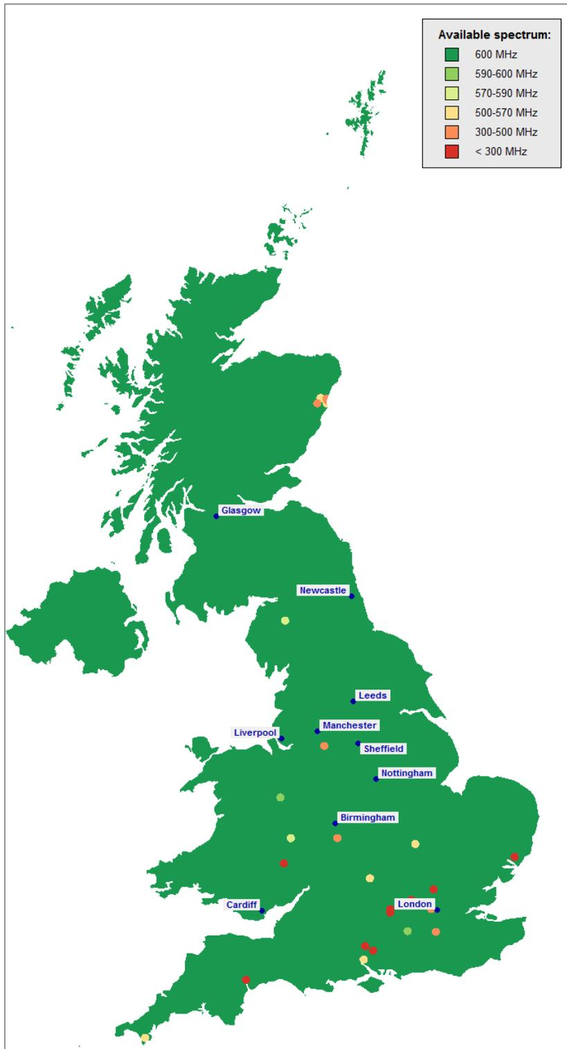
Figure A-17: Amount of spectrum (within the 3600 – 4200 MHz range) that could be available for IMT small cell use outdoors within the coordination areas around fixed link receivers based on ITU-R criteria
