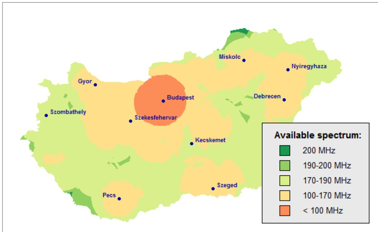
Figure A-3: Amount of spectrum (within the 3800 – 4200 MHz range) that could be available for IMT macro-cell use within the coordination areas around P-P fixed link receivers based on ITU-R criteria
