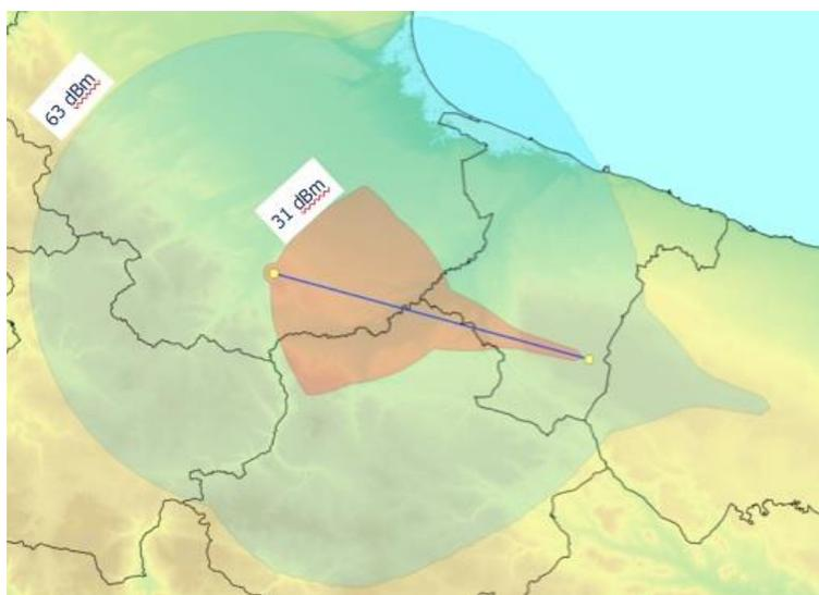
Figure A-11: FS link vs IMT transmitter exclusion zones
