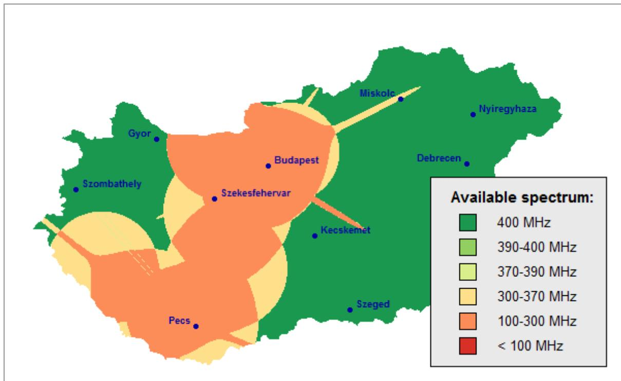
Figure A-4: Amount of spectrum (within the 3800 – 4200 MHz range) that could be available for IMT small cell use within the coordination areas around P-P fixed link receivers based on ITU-R criteria
