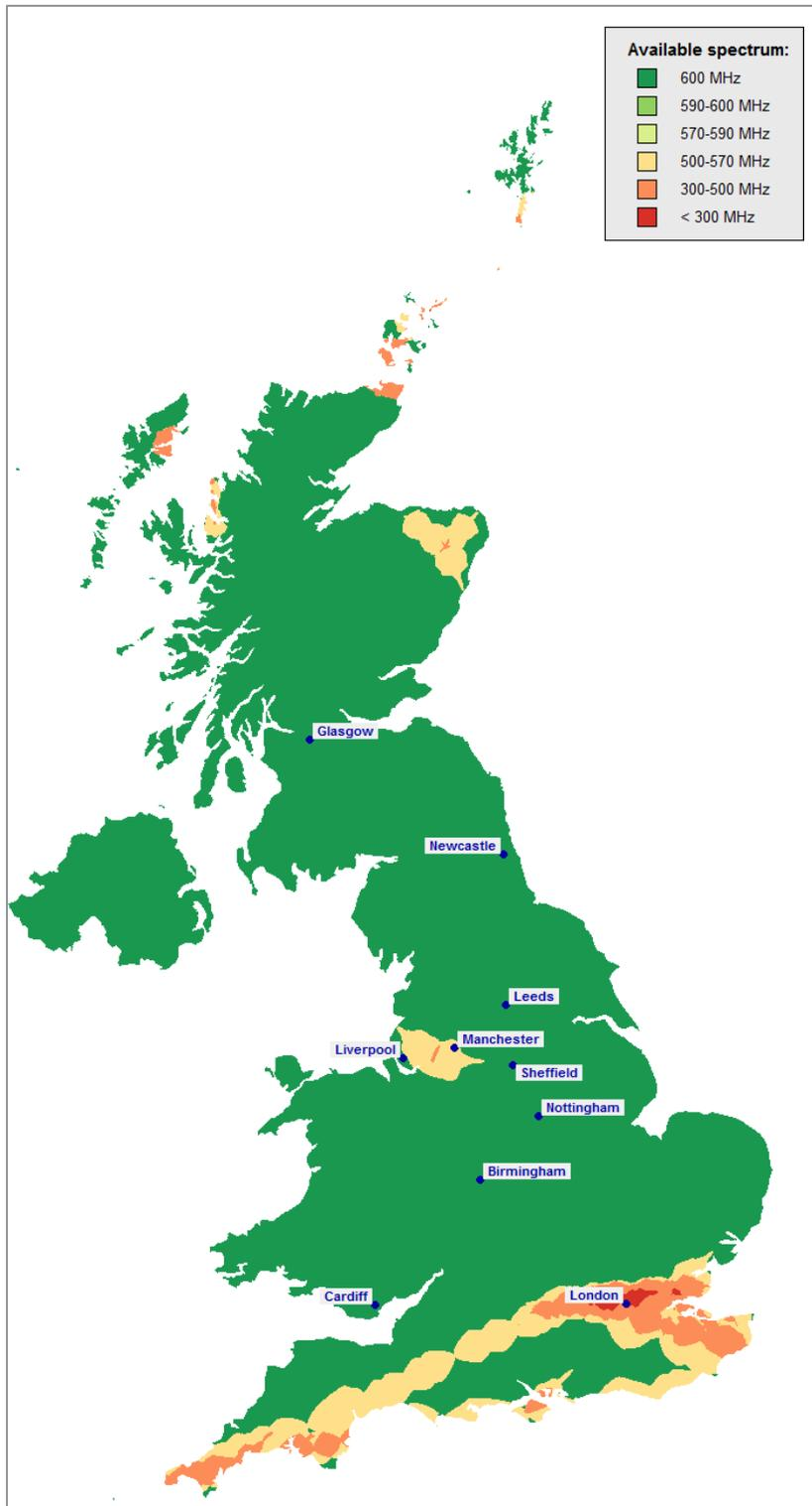
Figure A-18: Amount of spectrum (within the 3600 – 4200 MHz range) that could be available for IMT small cell use outdoors within the coordination areas around earth station and fixed link receivers combined based on ITU-R criteria
