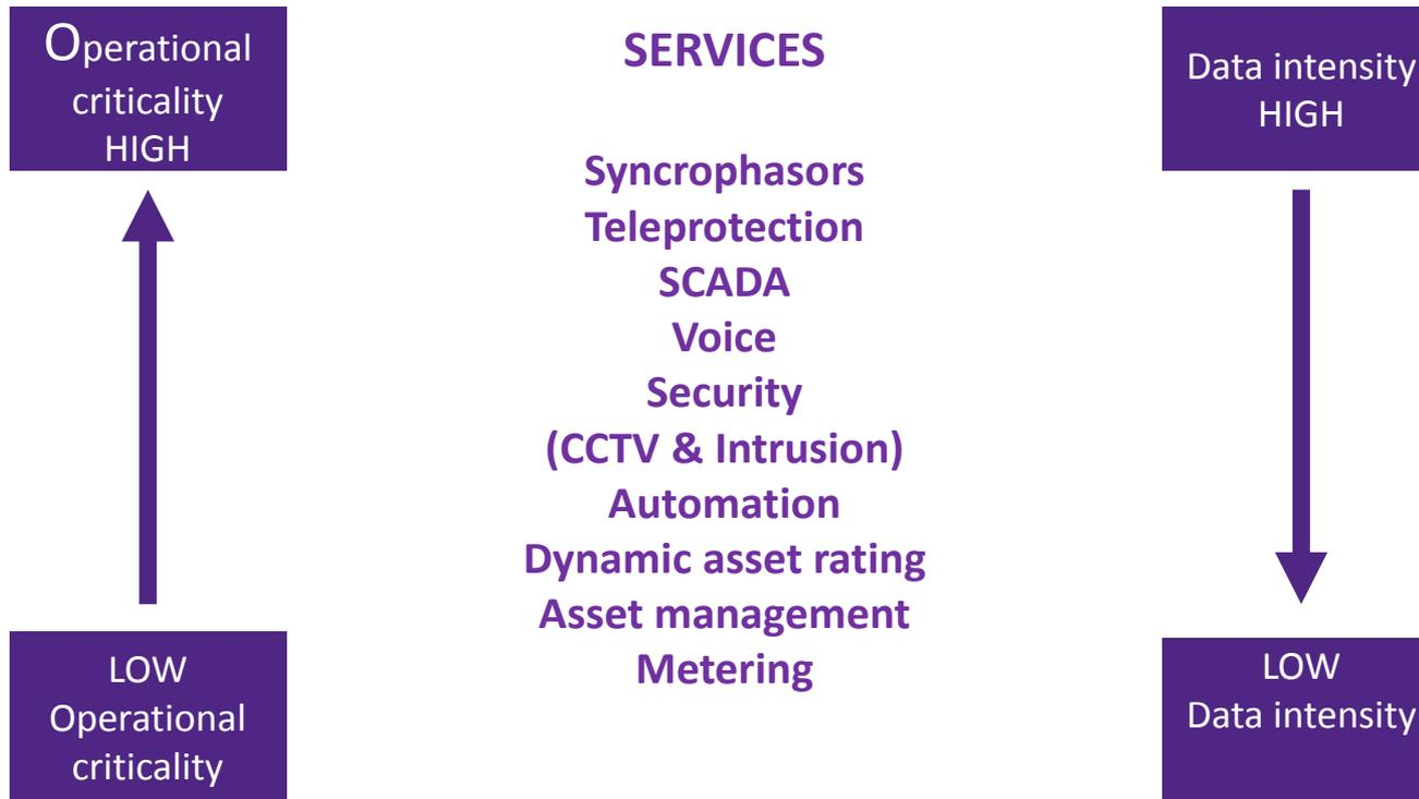
IEC 61850 – design of electrical substation automation defines latency requirements by mapping protocols on IP networks. Requirement of total transmission time < 4ms for protective relaying (trips and blocking) and  $\leq 10$  ms for releases and status changes.
