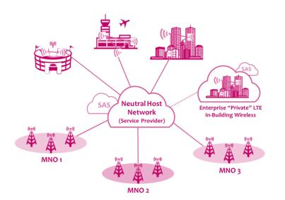
Figure 2.3: Neutral host network provider / Large enterprise LTE network using CBRS
