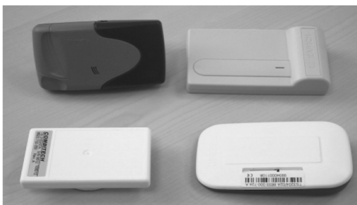
Figure A.2 – On board unit when microwave technology is deployed
