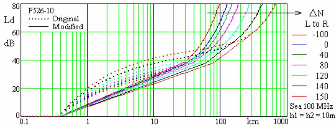
Figure 1-3. P526 original and modified spherical-earth model
