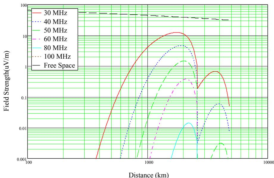
**Figure 1-2: Sporadic E field strength 1% time for Europe for a 1kW EIRP transmission**
