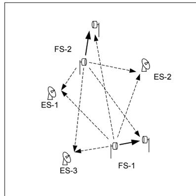
**Figure 7: Interference paths for example FS-ES deployment**
