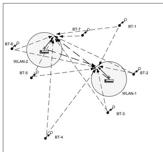
**Figure 8: Interference paths for example WLAN-BT deployment**
