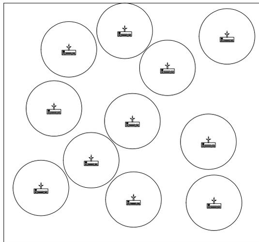
**Figure 9: Random deployment of WLANs**
