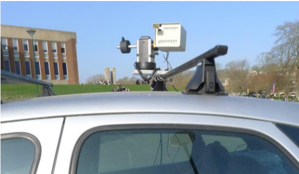
Figure 3: Receive down-converter on scanning mount
