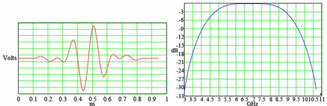
**Figure 4.1 : Example Wavelet and Its Spectrum**
