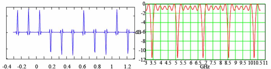
**Figure 4.2 : Example Code Sequence in Time and Frequency Domain
