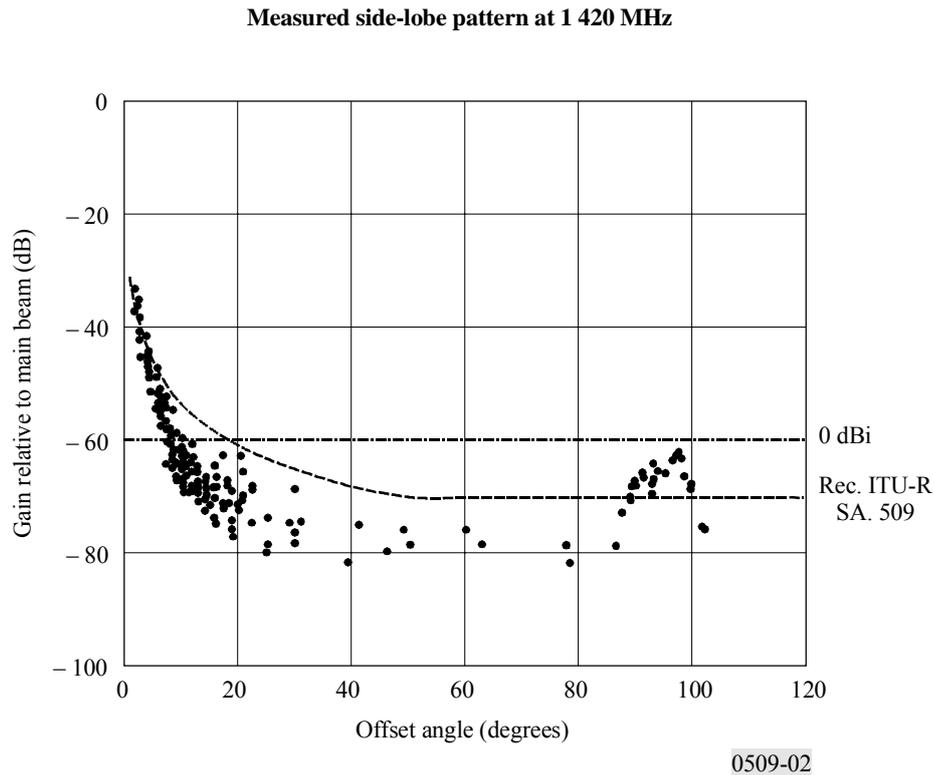
**Figure 3.6: Lovell telescope sidelobe measurements**
