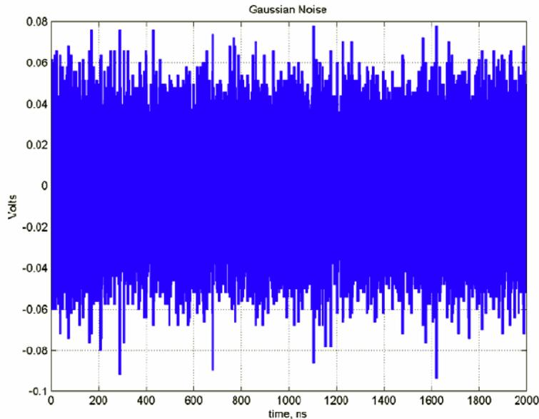
**Figure 4.9 : Gaussian Noise Emission in the Time Domain**
