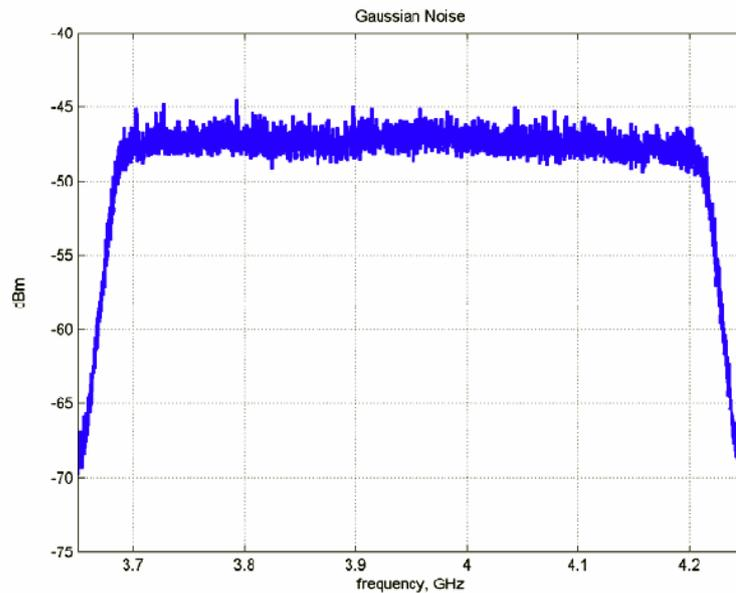
**Figure 4.8 : Spectrum Plot of Gaussian Noise**
