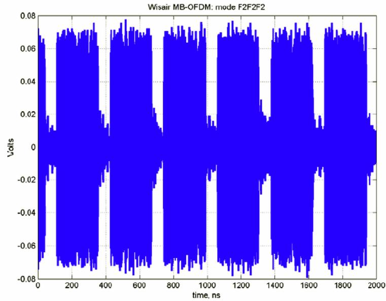
**Figure 4.14 : MB-OFDM Emission in A Non-Hopping Mode in the Time Domain
