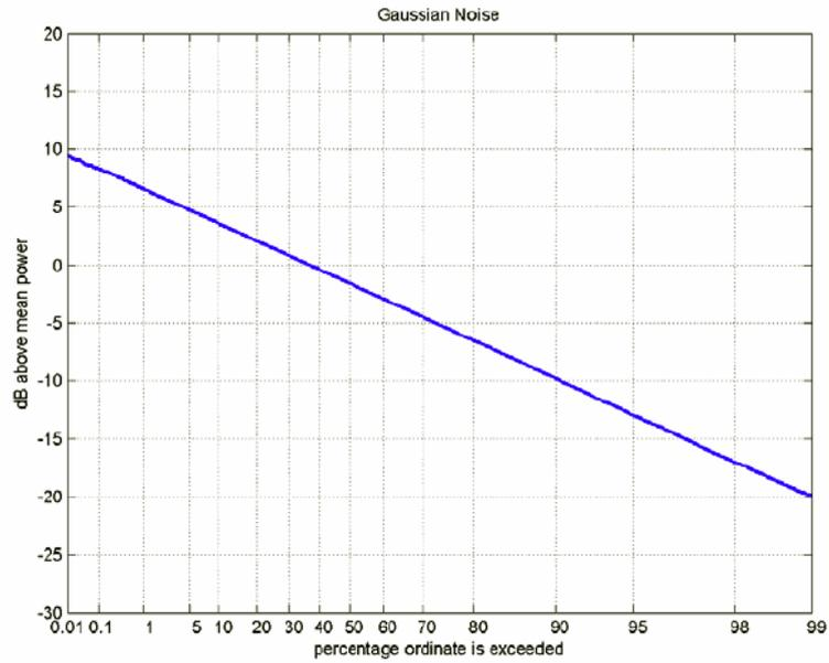
**Figure 4.7 : APD in 36 MHz Bandwidth of Gaussian Noise
