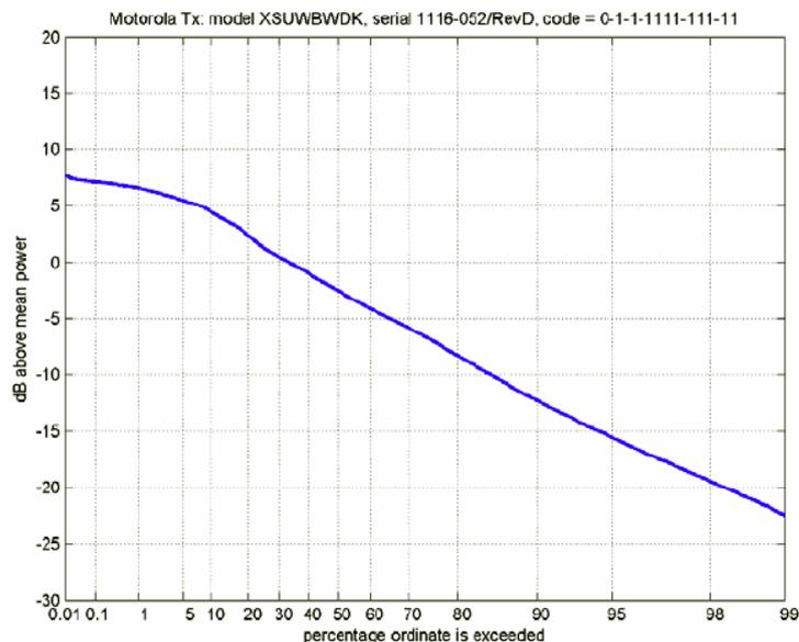
**Figure 4.4 : APD in 36 MHz Bandwidth of DS-UWB Emission (TX Designed to Operate In The Lower Band (3.1–4.85 GHz) with BPSK Modulation and Code Length 12)**
