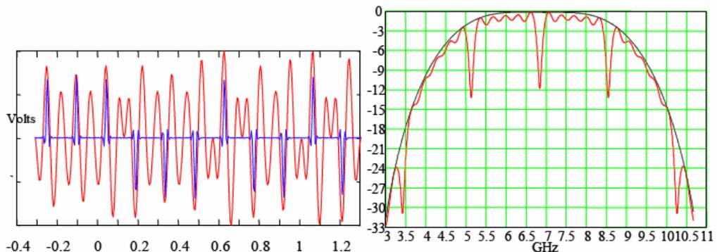
**Figure 4.3 : Example DS-UWB signal in Time and Frequency Domain
