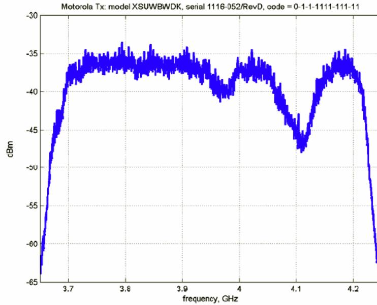
**Figure 4.5 : Spectrum Plot of DS-UWB Emission**
