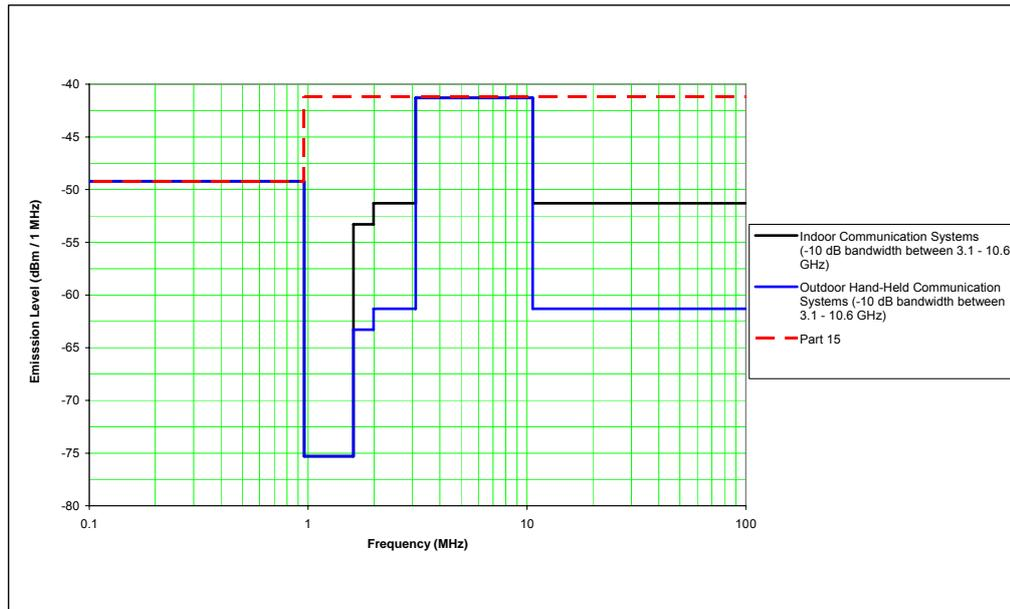
**Figure 2.1: FCC mask for UWB devices**
