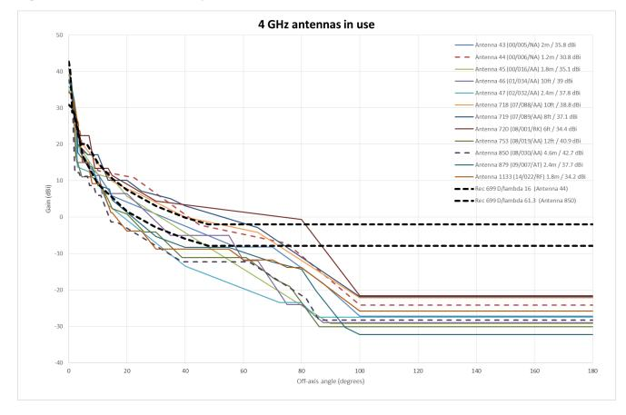
Figure A-23: Fixed link antenna patterns
