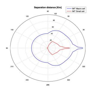
Figure A-9: FS receiver vs IMT transmitter exclusion zones
