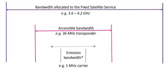
Figure 2-1: Relationship between different types of bandwidth
